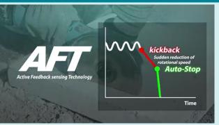
Active Feedback sensors (AFT), mechanical brake, anti-restart, and soft start.
